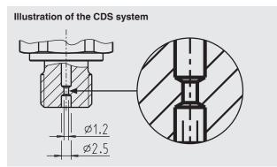
Fig. 1: Reduced diameter of the pressure channel
